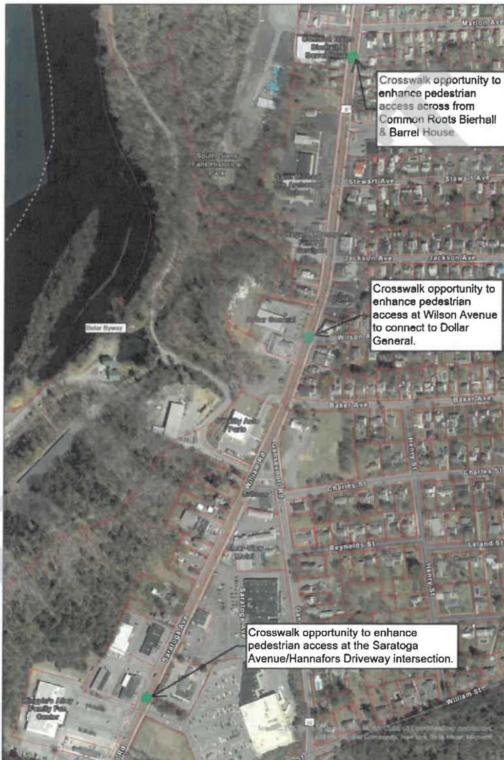
Figure 3. Recommended Locations for Crosswalk Installation
